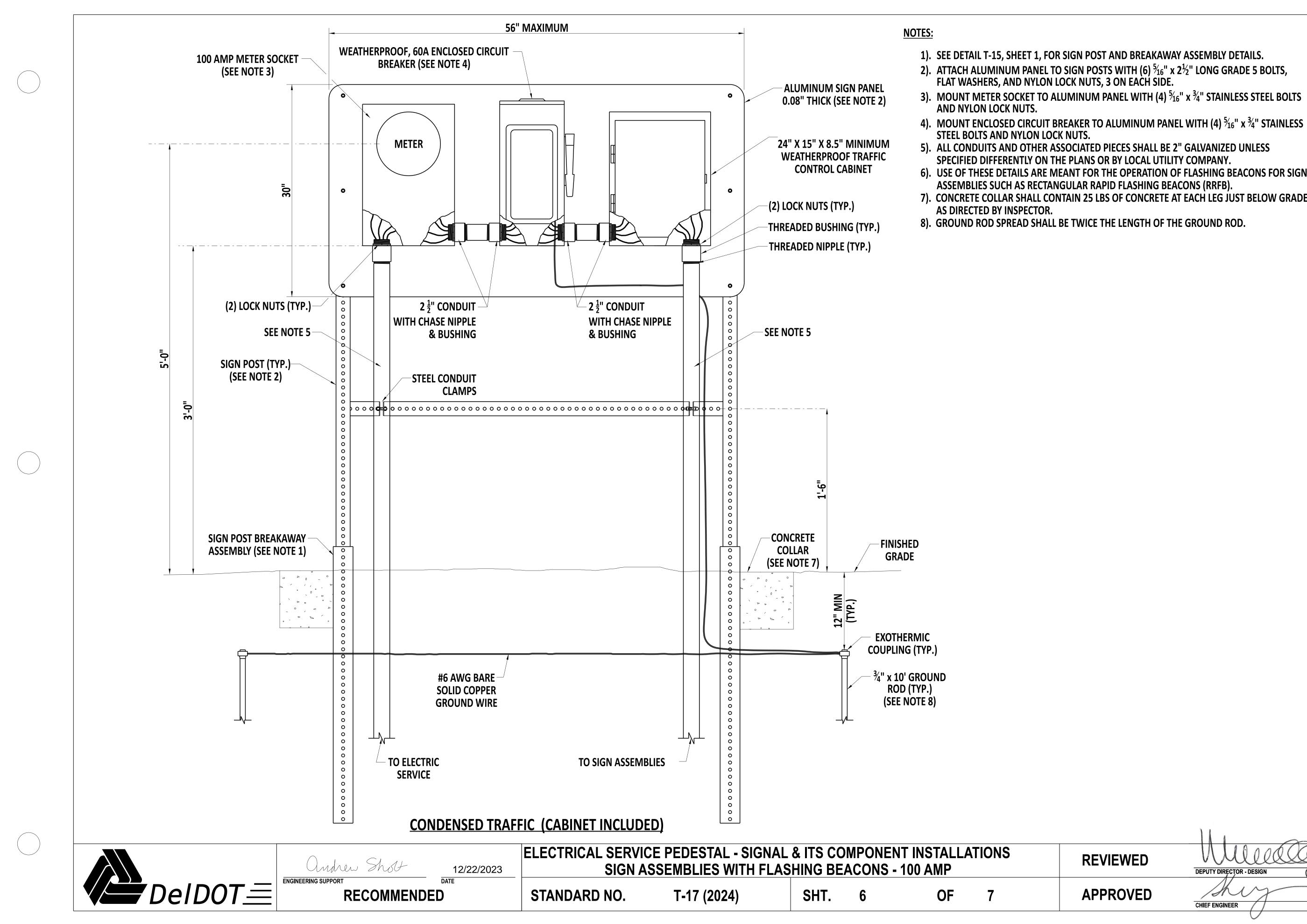
2). ATTACH ALUMINUM PANEL TO SIGN POSTS WITH (6)  $\frac{5}{16}$ " x  $2\frac{1}{2}$ " LONG GRADE 5 BOLTS, FLAT WASHERS, AND NYLON LOCK NUTS, 3 ON EACH SIDE.
