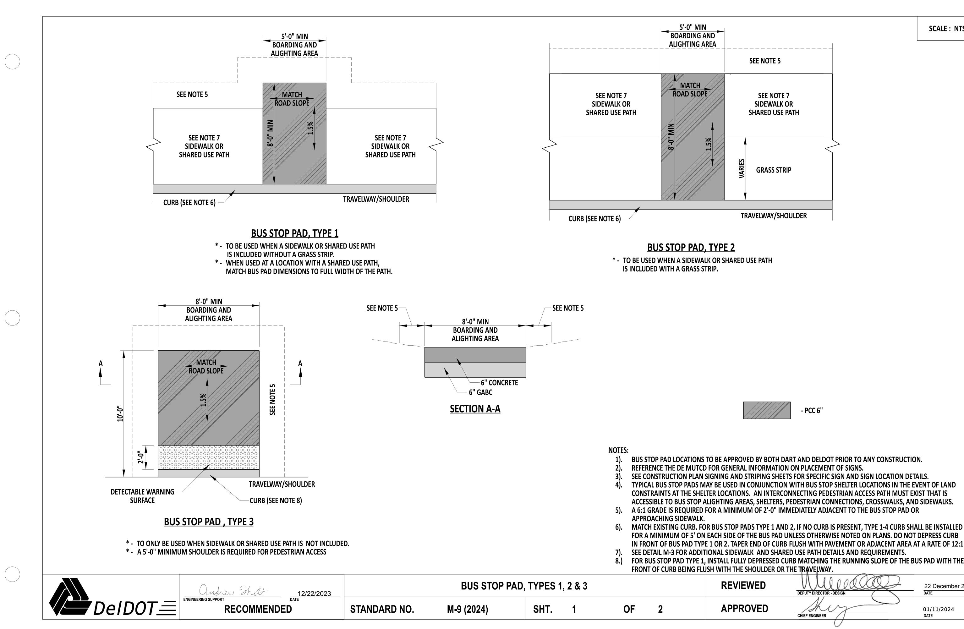
FOR A MINIMUM OF 5' ON EACH SIDE OF THE BUS PAD UNLESS OTHERWISE NOTED ON PLANS. DO NOT DEPRESS CURB IN FRONT OF BUS PAD TYPE 1 OR 2. TAPER END OF CURB FLUSH WITH PAVEMENT OR ADJACENT AREA AT A RATE OF 12:1. FOR BUS STOP PAD TYPE 1, INSTALL FULLY DEPRESSED CURB MATCHING THE RUNNING SLOPE OF THE BUS PAD WITH THE
